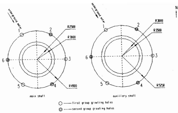
Figure 1. The locations of grouting holes
