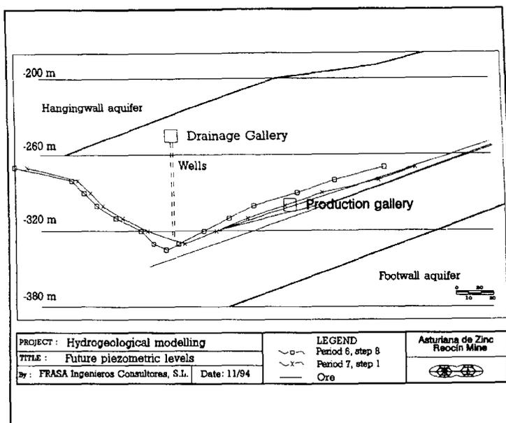
Figure 3. Mine drainage proposed at Reocin Mine, Spain (FRASA, 1994).
