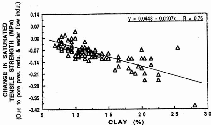
**Figure 5 - Change in saturated tensile strength due to pore pressure reduction and water flow induction vs percentage clay-sized fraction**
