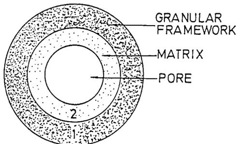
**Figure 2 - Conceptual model of cylindrical capillary**
