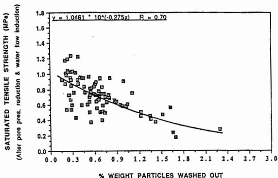
**Figure 4 - Saturated tensile strength after pore pressure reduction and water flow induction vs percentage of weight of particles washed out**
