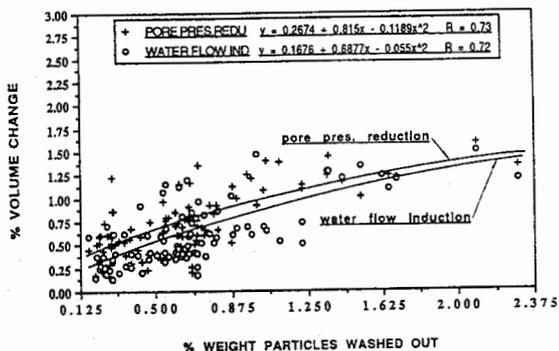
**Figure 1 - Percentage of volume change vs percentage of weight of particles washed out**
