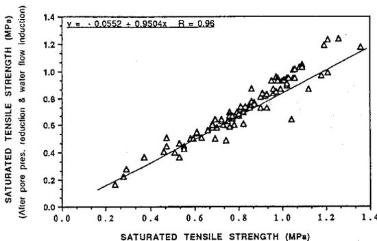
**Figure 3 - Saturated tensile strength after pore pressure reduction and water flow induction vs saturated tensile strength**
