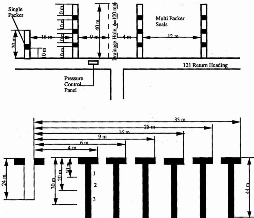
**Figure 4 Test arrangement to determine drainage influence**
