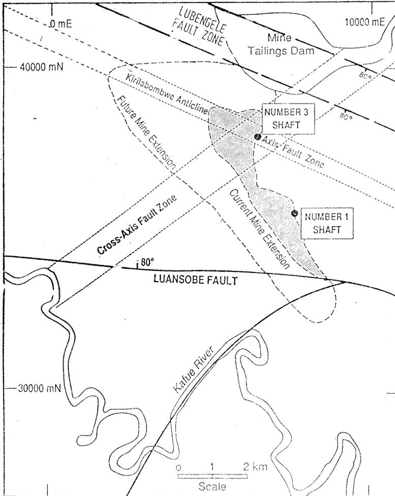
Fig. 4.1 : Map of Konkola Mine showing the faults, river, dam, and approximate limits of mining
