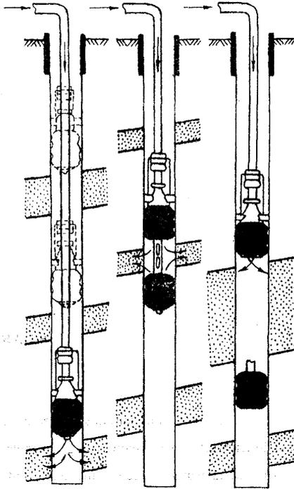
Fig.3 Technological scheme of grout injection.
