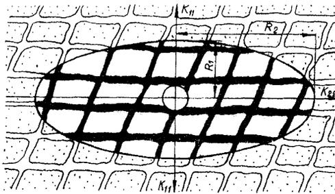
Fig.6 Sealing curtain design scheme for fractured rock.
