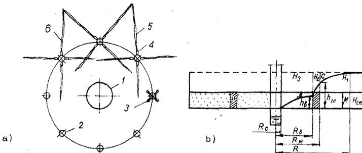
Fig.7 Sealing curtain design scheme for porous rock.
