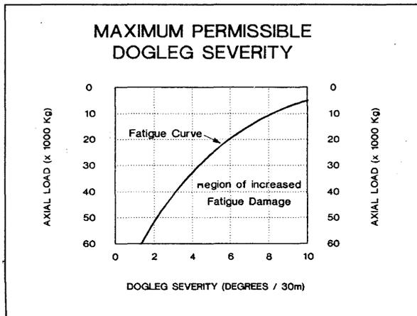
Figure 1.2 Typical fatigue curve for determining Maximum permissible dogleg severity
