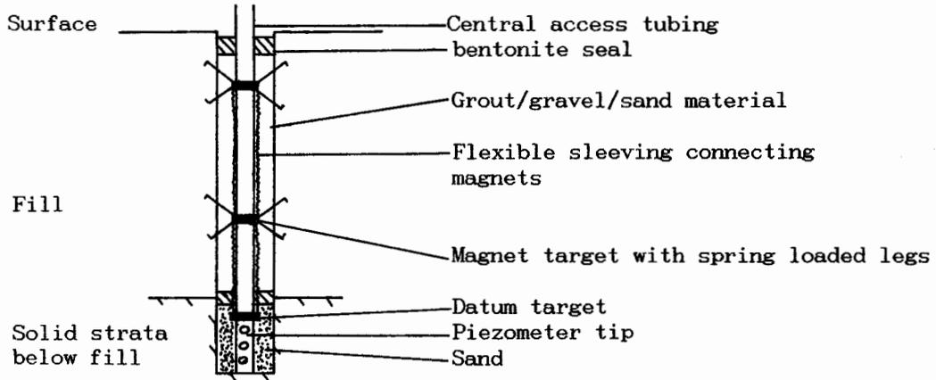
**Figure 6. The Magnetic Extensometer/Piezometer Instrument**
