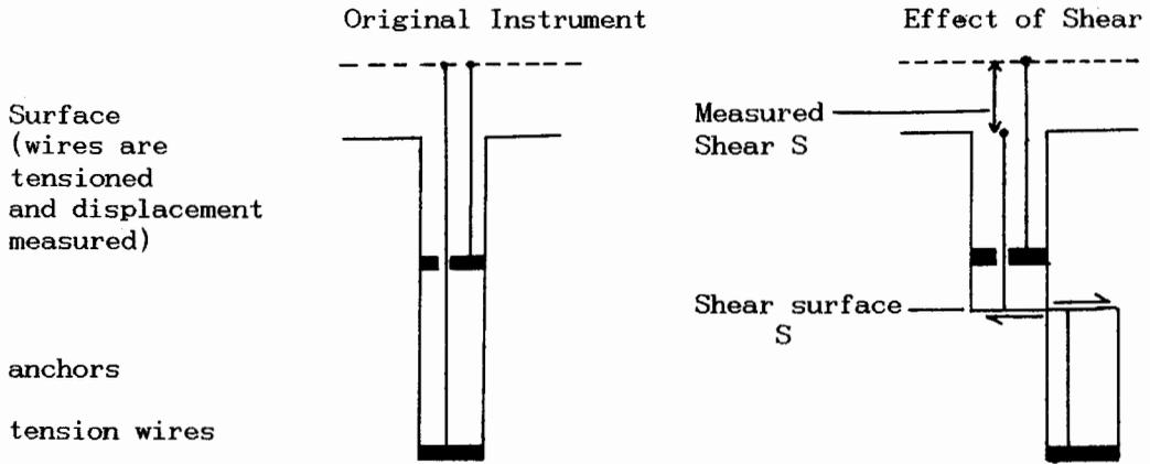
Figure 2. Measurement of shear by TWE
