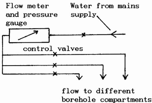
Figure 3. Testing Manifold
