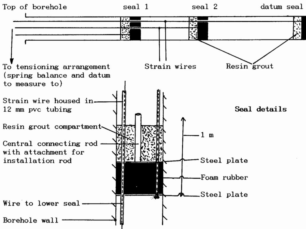
Figure 1. General details of the TWE with modifications for permeability testing.
