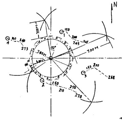
Fig.1 Geometry of grout hole pattern and deviation plan
