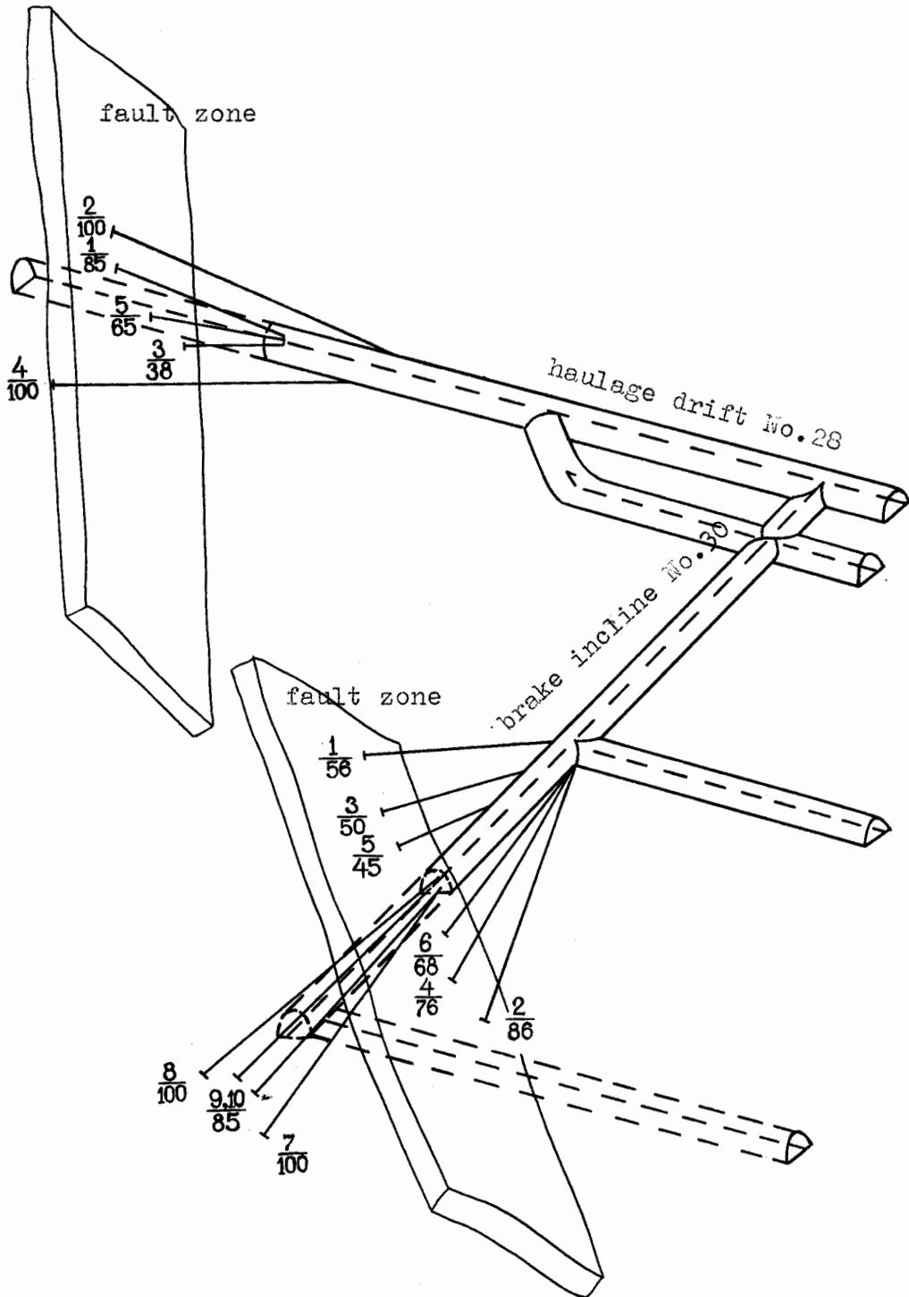
Fig. 2 Pregrouting procedure in driving development workings
