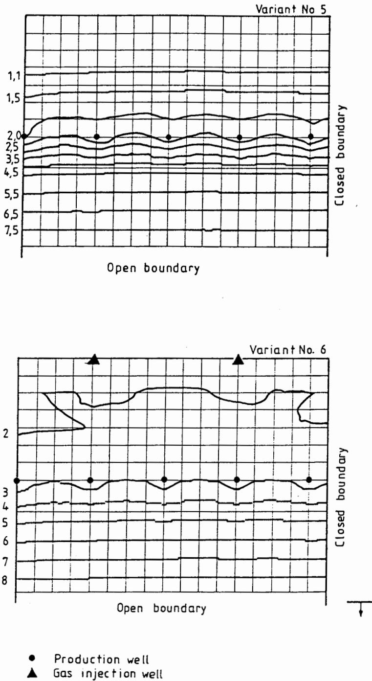
Water head maps of inclined variants at simulation time of 220 days [in bars]
