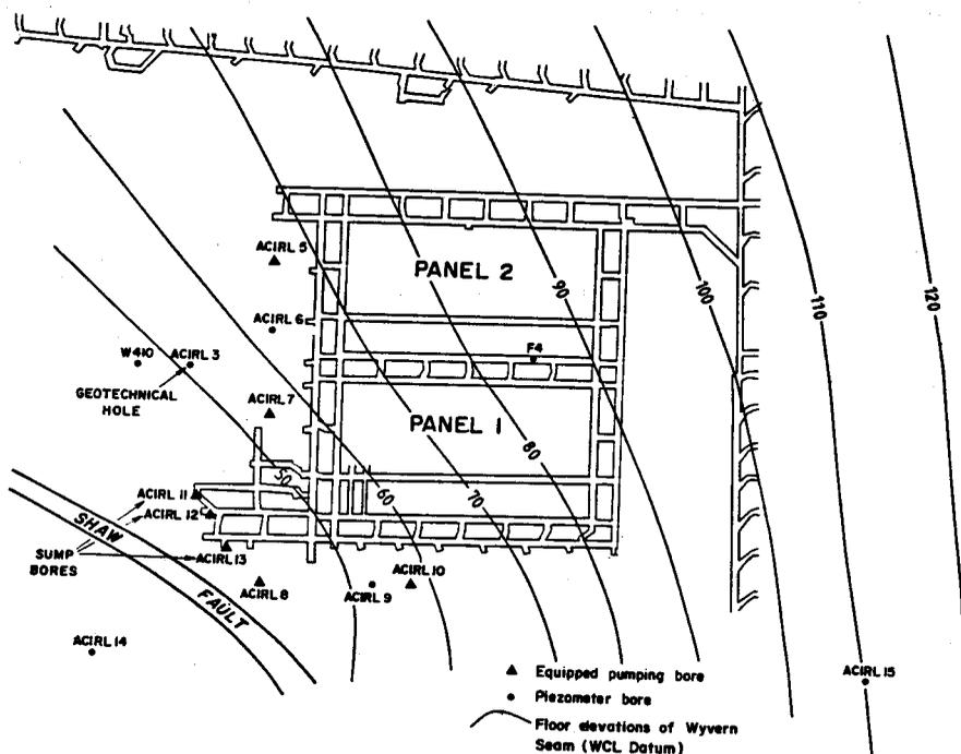
Figure 4 - Dewatering Bore Layout
