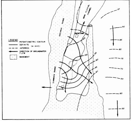
FIGURE 4 - GROUNDWATER FLOW AND RECHARGE SYSTEM
