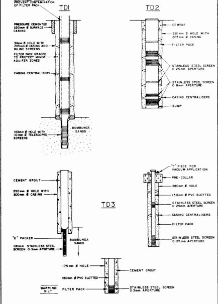
FIGURE 6 - DEPRESSURISATION BORE CONSTRUCTION DETAILS
