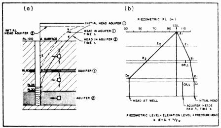
FIGURE 7 - MECHANISM FOR DEPRESSURISATION
